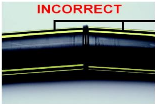
Pipe angled into fusion unit
