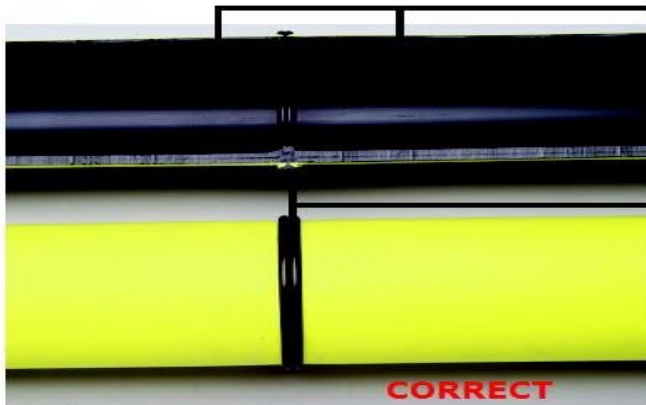
Proper double roll-back bead Proper alignment
