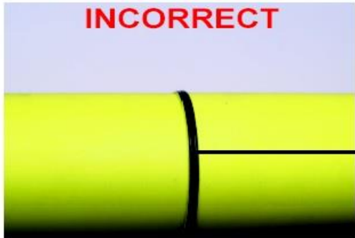
Insufficient heat time; melt bead too small
