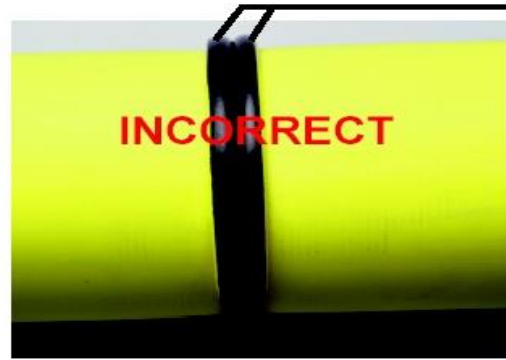
Excessive heat time or pressure applied during heating; melt bead too large
